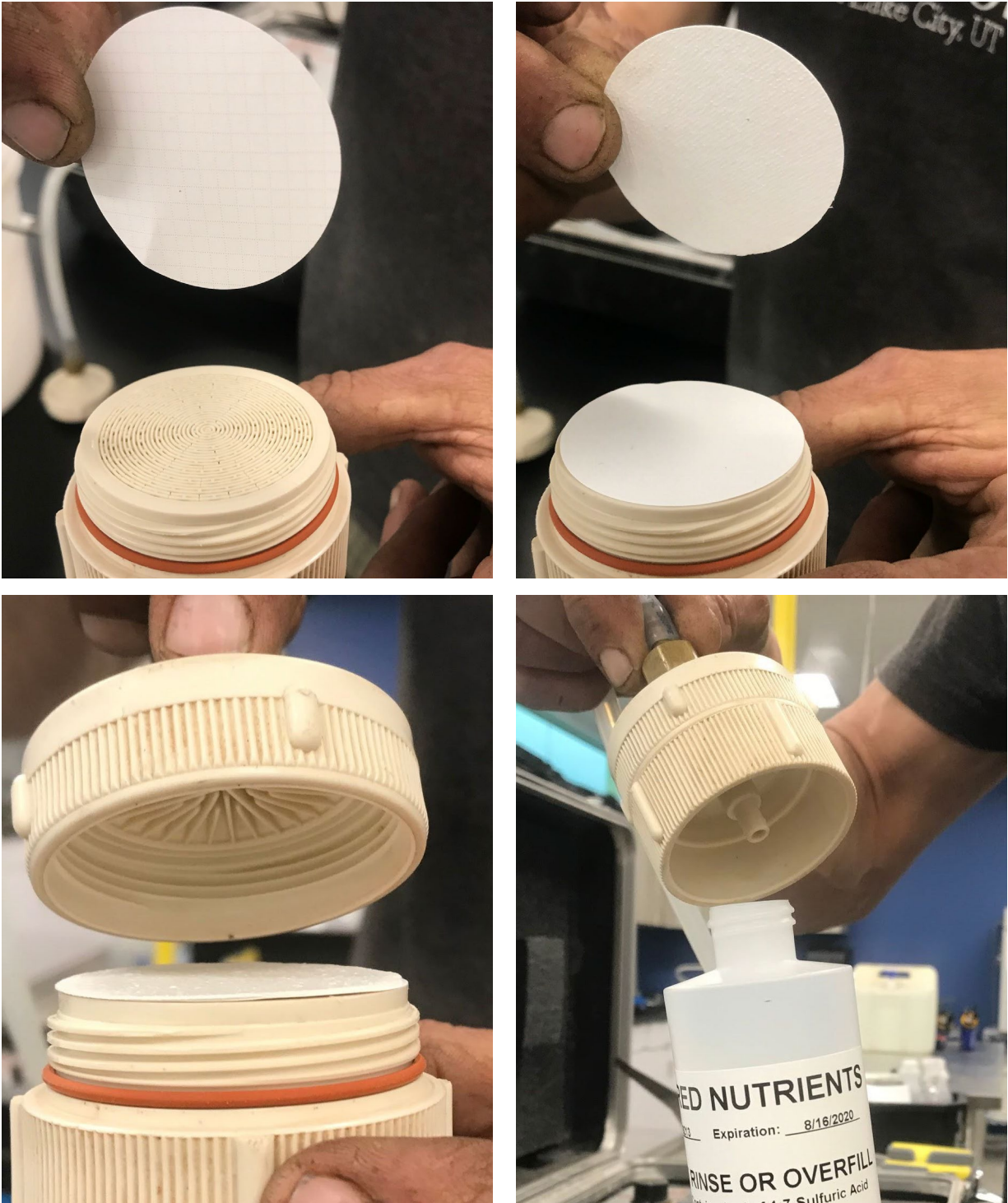
Figure 1: Membrane Filter Set-up: Gridded side down.
